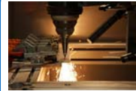
Laser welding in overlap position
